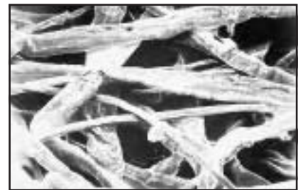
When all mechanisms are combined and utilized by a deep bed of the correct type of filter material, removal of virtually all particles whether liquid or solid, is achieved.
