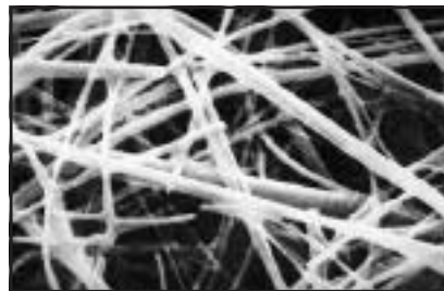
Above: Clean borosilicate microfiber seen at a magnification factor of 3900. Right: The same filter material in a contaminated state at the same degree of magnification.
